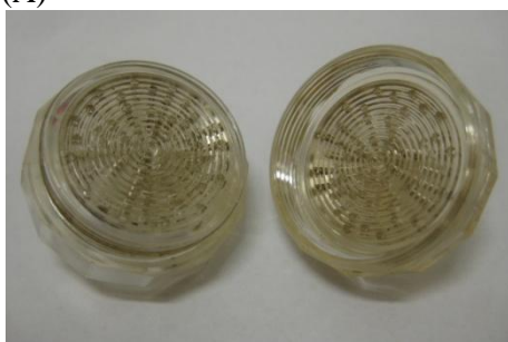
Fig. 5 Opened filterholder (A) and the toppart of filterholder with disassembled grid (B).
