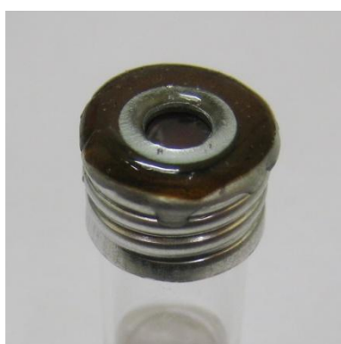
Fig. 10 Membrane glued with epoxy together with a lining disk to keep the epoxy away from the membrane over the hole.
