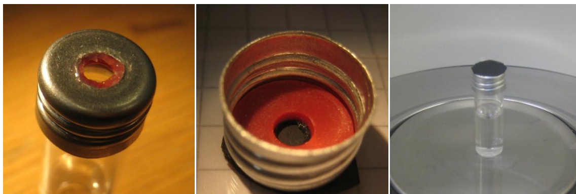
Fig. 9 Evaporation vial: (A) cap with open hole, (B) bottom view of cap, (C) vial, ready for measurement, with membrane glued on top and liquid inside.
