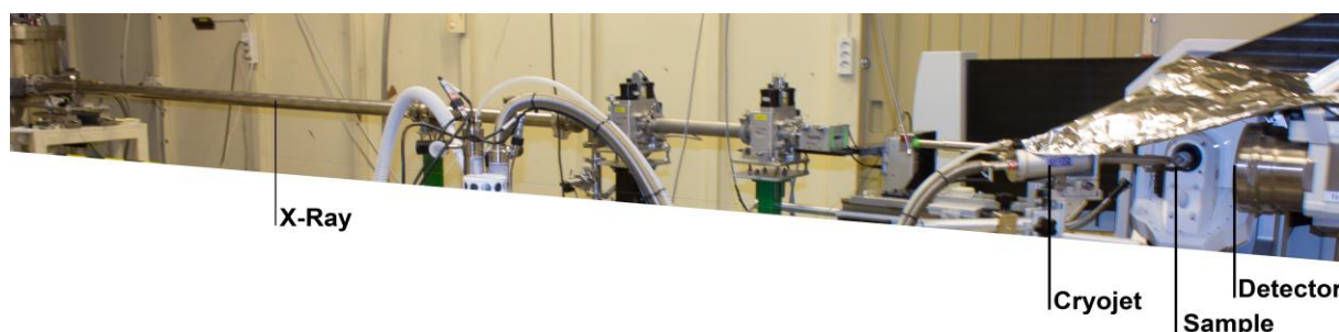
Fig. 21 Experimental setup at Beamline 711 for XRD measurements.
