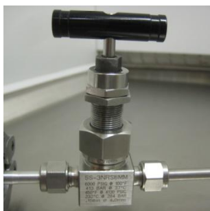
Fig. 4 Valve used for controlling the flow rate of the vacuum pumping.
