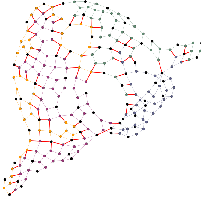
Figure 4.5: The STP instance eil101fst partitioned based on an edge-cut for k = 4 and d = 1.1 . This parameter choice for d clearly shows that without too much freedom in partition imbalance, the algorithm cannot find good partitions.
