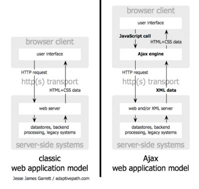
**Figure 3.2:** The traditional model for web applications (left) compared to the AJAX model (right). [14]
