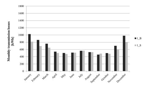
Figure 3-5 Monthly transmission losses based on dynamic thermal simulations in the brick building and in the virtual straw-bale building
