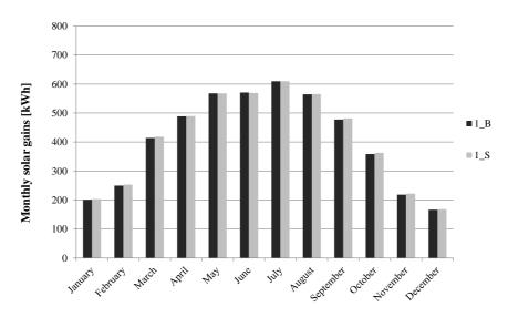
Figure 3-11 Monthly solar gains based on dynamic thermal simulations in the brick building and in the virtual straw-bale building
