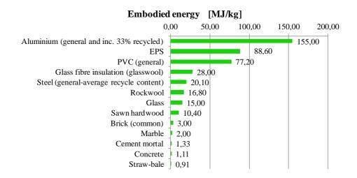
Figure 1-4 Embodied energy of different materials according to Greenspec EPDs (Greenspec 2013)
