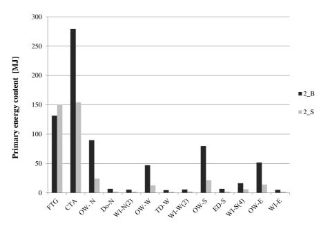
Figure 3-21 Primary energy content of different building elements based on OI3 indicators in the straw-bale building and in the virtual brick building
