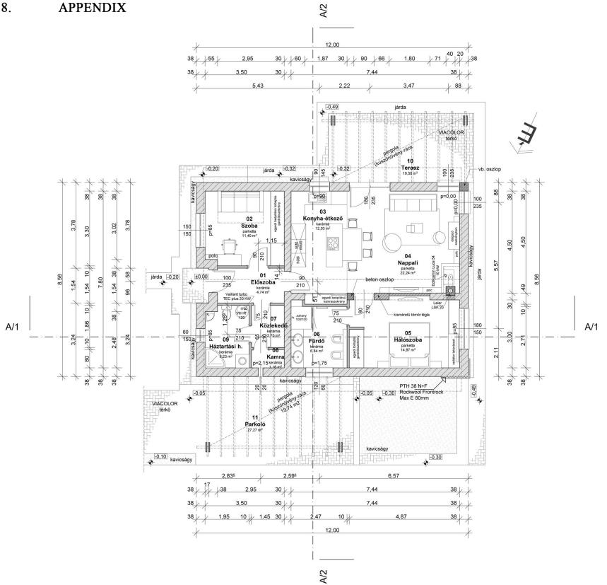
Figure 8-1 Plan of the brick building
