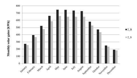
Figure 3-12 Monthly solar gains based on dynamic thermal simulations in the straw-bale building and in the virtual brick building
