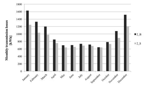
Figure 3-6 Monthly transmission losses based on dynamic thermal simulations in the straw-bale building and in the virtual brick building
