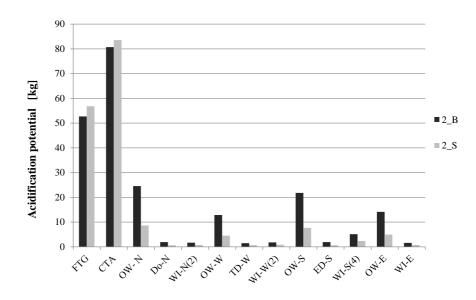
Figure 3-18 Acidification potential of different building elements based on OI3 indicators in the straw-bale building and in the virtual brick building
