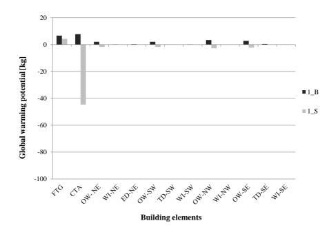
Figure 3-14 Global warming potential of different building elements based on OI3 indicators in the brick building and in the virtual straw-bale building
