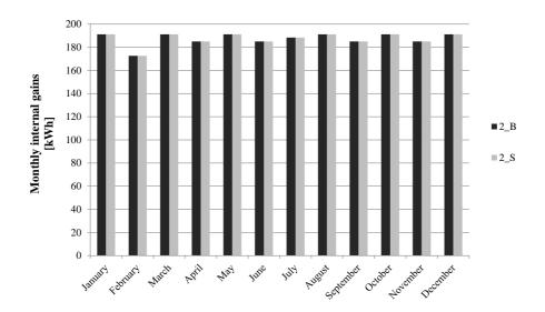
Figure 3-10 Monthly internal gains based on dynamic thermal simulations in the straw-bale building and in the virtual brick building
