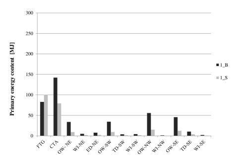
Figure 3-20 Primary energy content of different building elements based on OI3 indicators in the brick building and in the virtual straw-bale building
