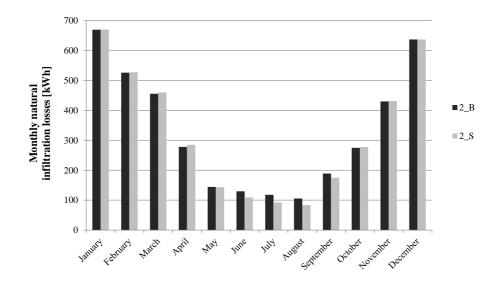
*Figure 3-8 Monthly natural infiltration losses based on dynamic thermal simulations in the straw-bale building and in the virtual brick building*
