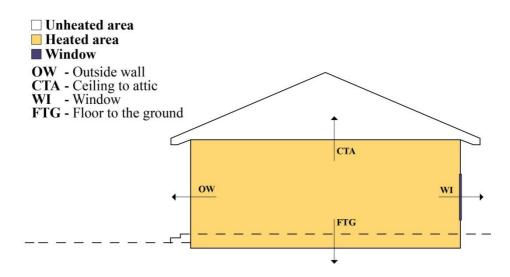
Figure 2-7 Building elements shown by location in the brick building and in the virtual straw-bale building
