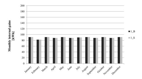
Figure 3-9 Monthly internal gains based on dynamic thermal simulations in the brick building and in the virtual straw-bale building
