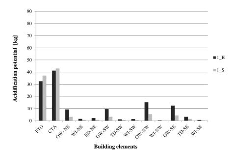
Figure 3-17 Acidification potential of different building elements based on OI3 indicators in the brick building and in the virtual straw-bale building
