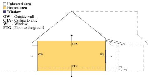
Figure 2-9 Building elements shown by location in the straw-bale building and in the virtual brick building
