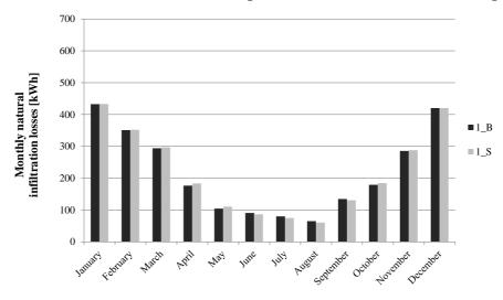
Figure 3-7 Monthly natural infiltration losses based on dynamic thermal simulations in the brick building and in the virtual straw-bale building
