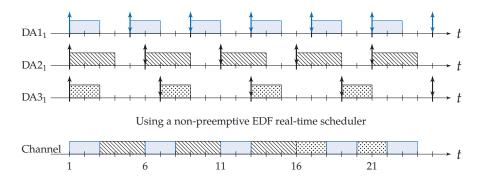
Figure 2.15: Messages generated by the three distributed algorithms on processing node 1 and how they get scheduled on the shared channel to another processing node.
