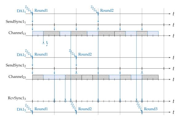
Figure 2.17: Detailed communication schema for sending messages within an execution of distributed algorithm DA1. Events and messages related to DA1 are colored.
