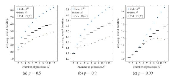
Figure 4.6: Monte-Carlo simulation results for case I compared against the calculated lower bound and the calculated expected round duration of case III serving as an upper bound.
