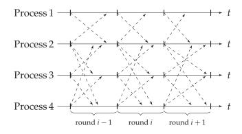
Figure 2.3: Example of a part of a synchronous execution as it could occur in the distributed system shown in Figure 2.2.
