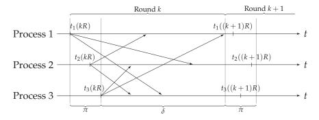
Figure 2.7: Generating rounds from approximately synchronized clocks.
