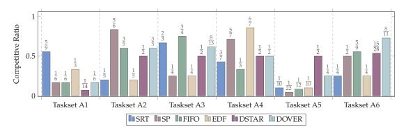
Figure 3.6: The competitive ratio of the examined algorithms in various tasksets under no constraints. Every examined algorithm is optimal in some taskset, among all others.
