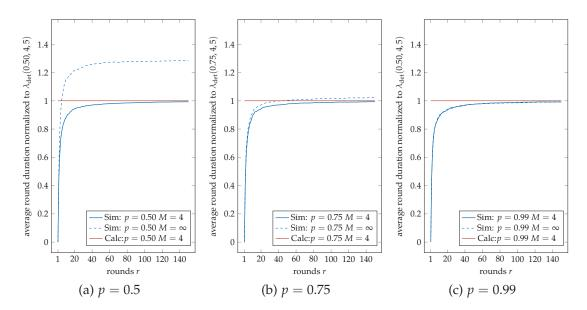
Figure 4.9: Simulated  $T_1(r)/r$  versus r for  $\mathcal{N} = 5$  and  $M = \{4, \infty\}$  in deterministic loop-back systems with  $p = \{0.5, 0.75, 0.99\}$ , normalized to  $\lambda_{det}(5, p, 4)$ .
