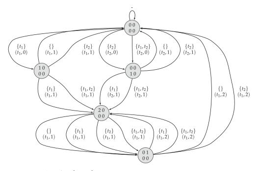
Figure 3.1: EDF for  $\mathcal{T} = \{\tau_1, \tau_2\}$  with  $D_1 = 3$ ,  $D_2 = 2$  and  $C_1 = C_2 = 2$ , represented as a deterministic LTS.
