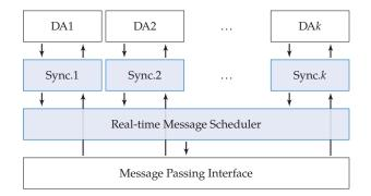
Figure 2.16: Layered structure of one node in the proposed system model, running processes of k independent distributed algorithms. Contributions of this thesis are colored.
