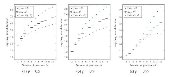
Figure 4.7: Monte-Carlo simulation results for case II compared against the calculated lower bound and the calculated expected round duration of case III serving as an upper bound.
