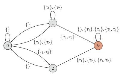
Figure 3.2: Example of a safety LTS  $L_S$  that restricts the adversary to release at most 2 units of workload in the last 2 rounds.
