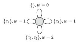
Figure 3.4: Example of a limit-average LTS  $L_W$  that tracks the average workload of jobs released by the adversary.
