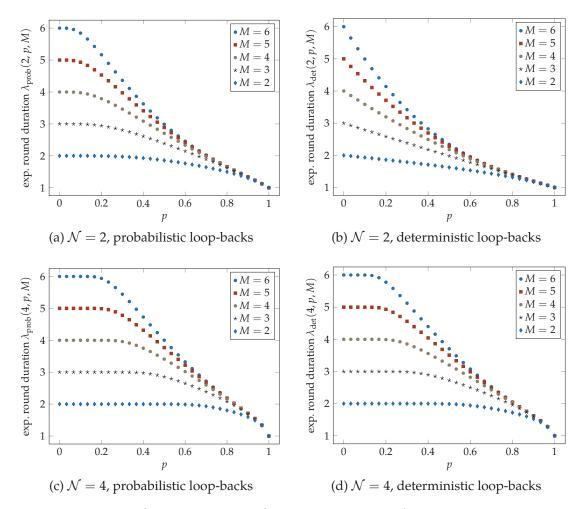
Figure 4.3:  $\lambda_{\text{prob}}(\mathcal{N}, p, M)$  and  $\lambda_{\text{det}}(\mathcal{N}, p, M)$  versus p for  $\mathcal{N} = \{2, 4\}$  and  $2 \leq M \leq 6$ .
