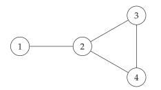
Figure 2.2: Example for the communication graph of a distributed system.
