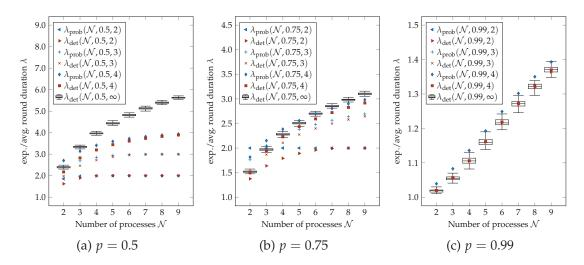
Figure 4.10:  $\lambda_{\text{prob}}$ ,  $\lambda_{\text{det}}$  for  $M \leq 4$  and simulations (deterministic loop-backs,  $M = \infty$ ) versus  $\mathcal{N}$  for  $p = \{0.5, 0.75, 0.99\}$ .
