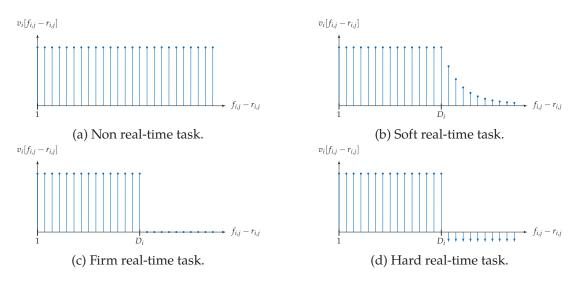
Figure 2.11: Time/utility functions of different kinds of real-time tasks.
