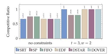
Figure 3.7: Restricting the absolute workload generated by the adversary typically increases the competitive ratio, and can vary the optimal scheduler. On the left, the performance of each scheduler is evaluated without restrictions: FIFO, SP behave best. When restricting the adversary to at most 2 units of workload in the last 3 rounds, FIFO and SP become suboptimal, and are outperformed by other schedulers.
