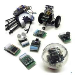
**Figure 2.5:** A Wide Field of Sun SPOT Applications: Robots, Remote Controls and Cybernetic Devices such as an Electronic Glove. Source: [ORACLE, 2012b].
