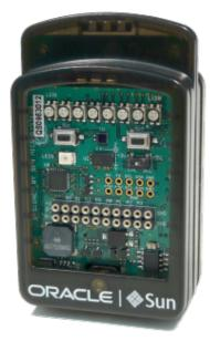
**Figure 2.3:** Front View of a New Sun SPOT with eDEMO Daughterboard. Source: [ORACLE, 2012b].
