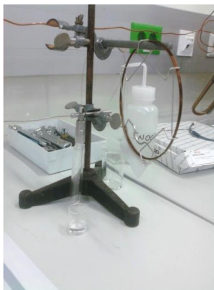
Figure 107: Apparatus for coating of capillary columns
