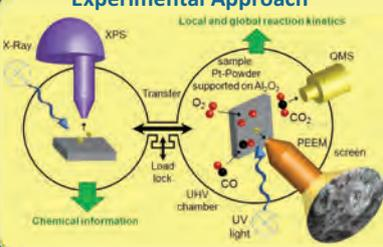
Local reaction kinetics was evaluated from the analysis of PEEM video-frames recorded *in situ* during the ongoing CO oxidation reaction in the  $10^{-5}$  mbar pressure range. The local image brightness is related via the work function to the local CO- or O-coverage and thus to the local  $\text{CO}_2$  production rate [4]. Simultaneously, the global  $\text{CO}_2$  reaction rate was measured by mass spectrometry (MS).
