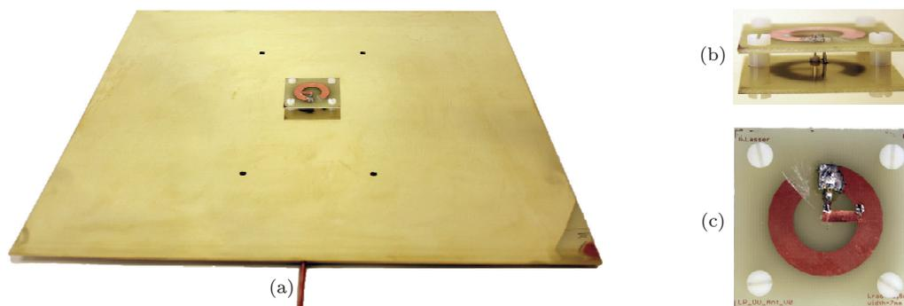
Figure 2.6: Image showing the LPDL antenna (a), and close-ups of the vertical feed (b), and the PCB (c).
