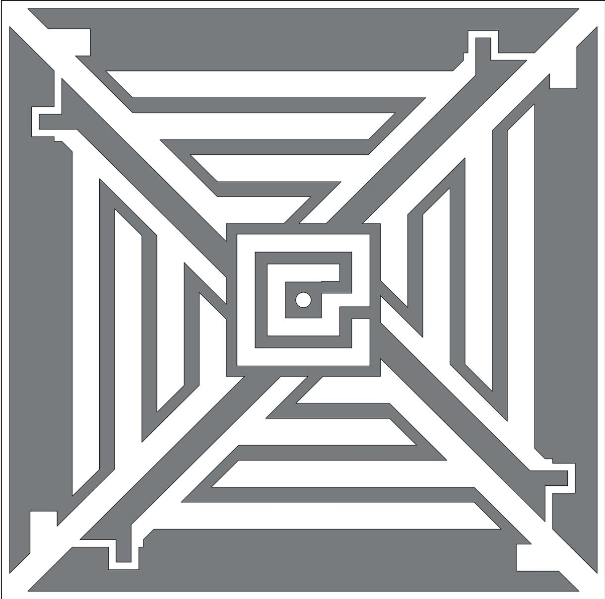
Figure B.2: Drawing of a unit cell of FSS FSS2 in scale 8:1. The thin boarder line corresponds to the 20 mm unit cell boundary.
