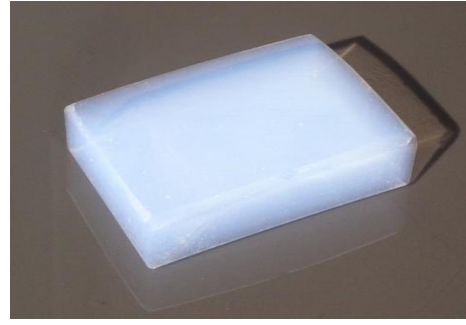
Figure 11. Scheme of aerogel (Illumina- Chemie 2008)
