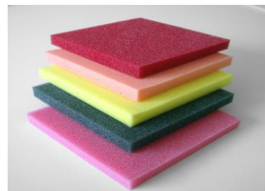
Figure 3. Scheme of polyurethane foam (Directindustry 2008)
