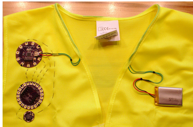
Figure 3.20: High visibility vest with added power circuitry
