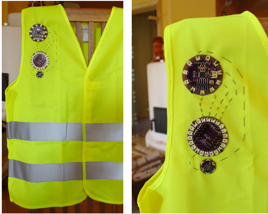
Figure 3.19: LilyPad components on a high visibility vest
