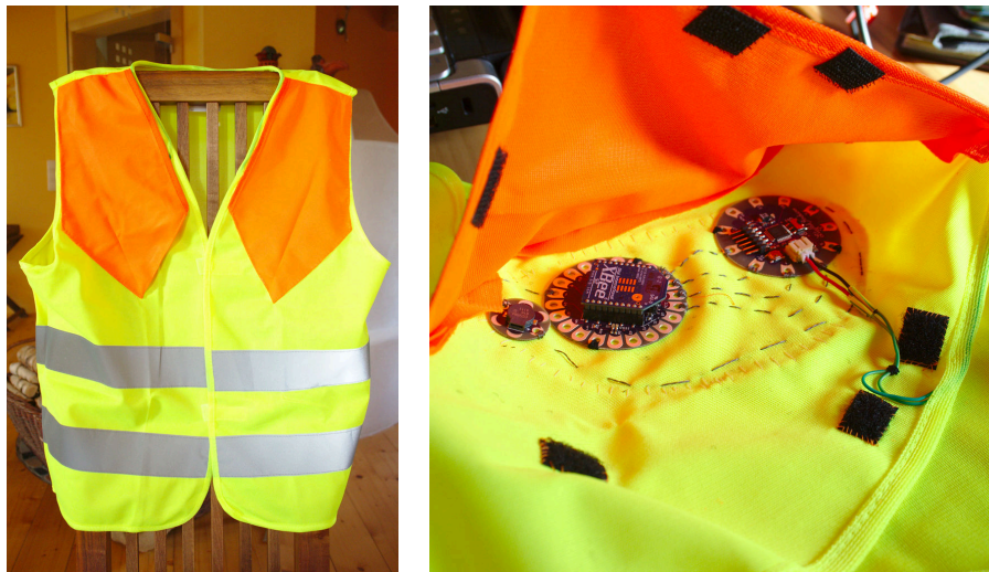
(a) fabric to cover the LilyPad (b) a peek at the electronics beneath
