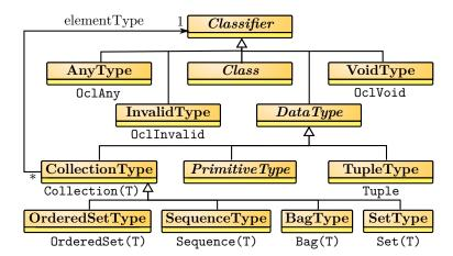
Figure 10: Partial OCL type hierarchy, adapted from [36]
