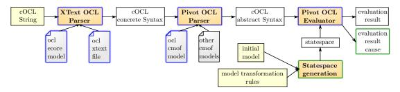
Figure 25: Architecture of the XText OCL plugin. Modified parts are highlighted blue, added parts green
