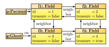
Figure 38: Partial object diagram of the initial field. All objects are contained in the game object
