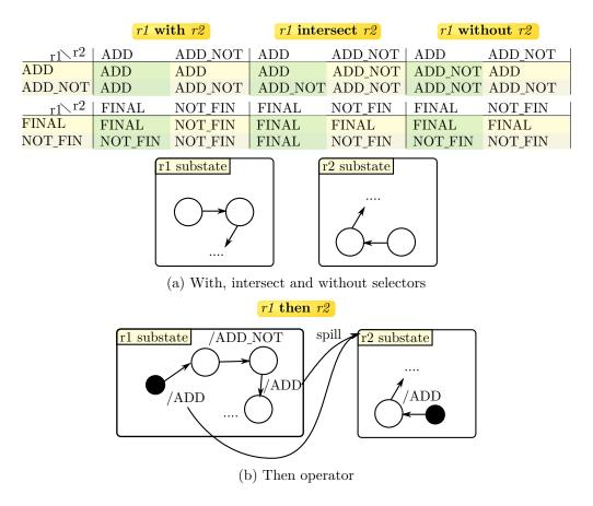
Figure 30: State diagrams for different compound selector operations
