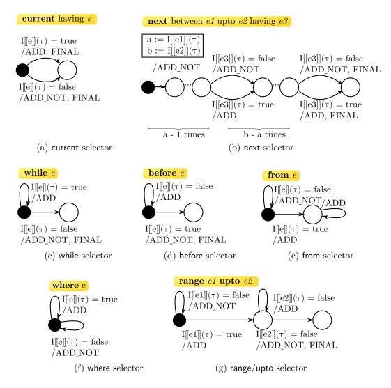
Figure 29: State diagrams for different primitive selector operations
