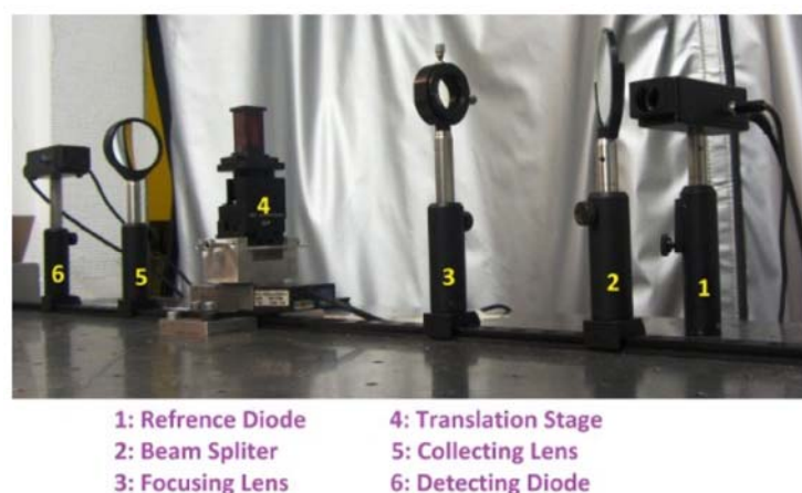
Fig 86 Scheme of the open aperture z-scan analysis 150
