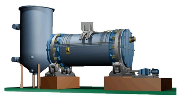
An example of an anode furnace (Kopar, 2010)
