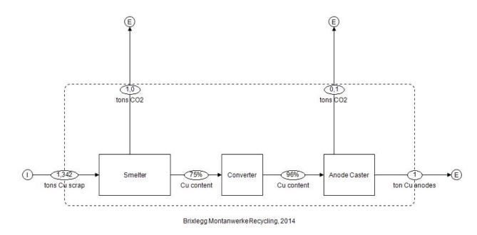
The material flow analysis for Brixlegg shows the amount of copper scrap needed to produce one tonne of copper annodes and the amount of the resulting carbon dioxide emissions. This is not meant to show mass balances but instead show an unbalanced flow diagram.
