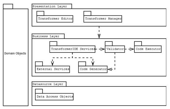
Figure 4-4 The three-tier architecture of the TransformerIDE
