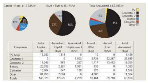
Figure 29: Cost breakdown of optimized Koh Pu system. Source: Graencen et al 2007, page 25.
