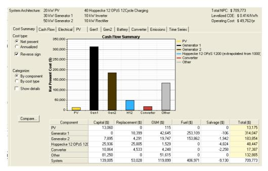
Figure 35: HOMER results for optimal hybrid system configuration in Optimization Exercise 1. Source: Own results.
