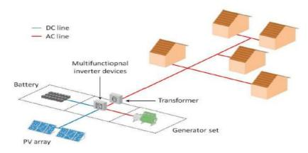
Figure 19: Schematic view of a PV/diesel hybrid system for rural electrification. Souce: IEA PVPS Task 09/CLUB-ER 2013, page 7.
