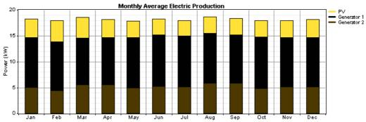
Figure 36: Monthly Average Electric Production for optimal hybrid system configuration in Optimization Exercise 1. Source: Own results.
