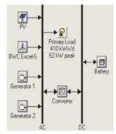
Figure 25: AC bus system has renewable sources directly connected to AC lines that go throughout the village. Source: Graencen et al 2007, page 16.
