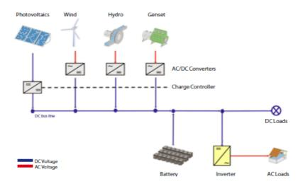
Figure 9: DC coupled power system. Source: ARE 2011, page 29.
