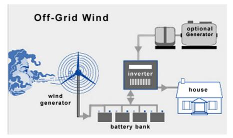
Figure 21: Off-Grid Wind System. Source: URL 6.
