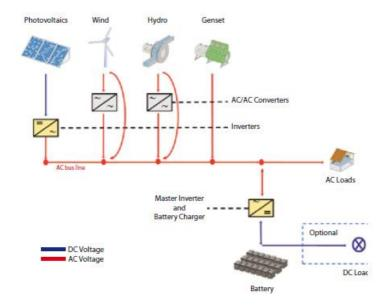
Figure 8: AC coupled hybrid power system. Source: ARE 2011b, page 28.
