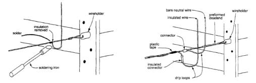
Figure 48: Soldering a twister copper to copper connection. | Figure 49: Connection between duplex service conductor and the residence. Source ESMAP 2000, page 152/153.
