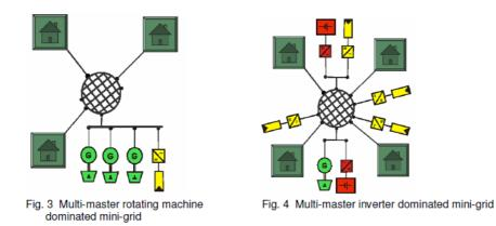
Figure 13: Multi-master rotating machine dominated mini-grid. | Figure 14: Multi-master inverter dominated mini-grid. Source: IEA/PVPS Task 11 2012, page 20.
