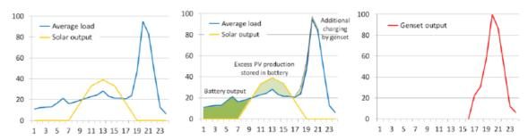
Figure 18: 70 kWp hybrid system in Cambodia: average daily load curve, solar output, battery and genset use (values in kW). Source: IEA PVPS Task 9/CLUB-ER 2013, page 9.
