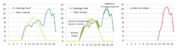
Figure 17: 16 kWp hybrid system in Mauretania: average daily load curve, solar output, battery and genset use (values in kW). Source: IEA PVPS Task 9/CLUB-ER 2013, page 9.
