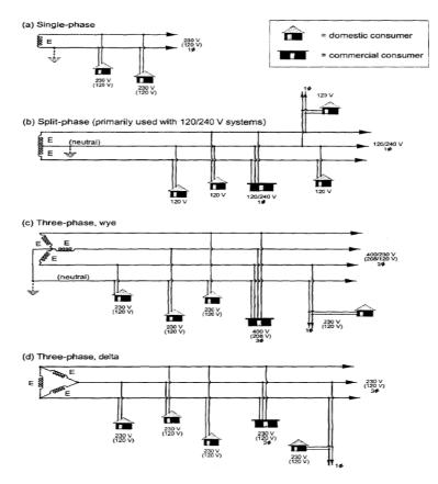
Figure 15: The four basic distribution line configurations that may have application for a village minigrid. E represents the commonly used voltage in the country (generally 120 V or 230 V). Source: ESMAP 2000, page 55.
