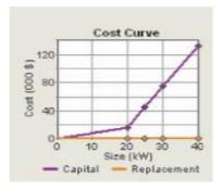
Figure 26: Cost curve for installed PV in Bahn Koh Pu. Replacement cost is irrelevant as no PV is replaced in the time period covered in the analysis (PV life and project life are both set at 20 years). Source: Graencen et al 2007, page 19.
