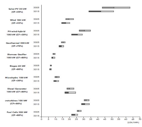
Figure 24: Mini-Grid Forecast Generating Cost. Source WB 2007, page 256.
