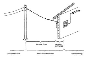
Figure 47: The basic components delivering power from the distribution line to the user. Source: ESMAP 2000, page 145.
