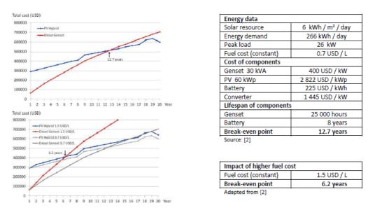
Figure 20: Example of 60 kWp PV/diesel hybrid system in Ecuador: simulation of total accumulated costs over 20 years. Source: IEA PVPS Task 09/CLUB-ER 2013, page 15 (taken from ARE 2011).
