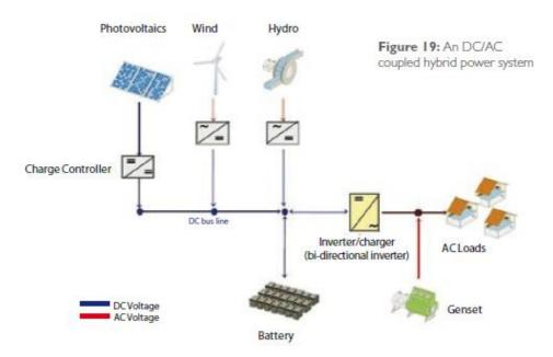
Figure 10: DC/AC coupled hybrid power system. Source: ARE 2011b, page 29.
