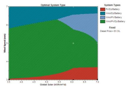
Figure 34: Optimal system type at different natural conditions with a fixed oil price at 1,30 USD per liter. Source: ARE 2011, page 18.
