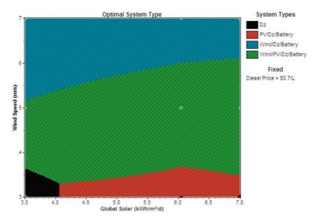
Figure 33: Optimal system type at different natural conditions with fixed oil price of 0,70 USD per liter. Source: ARE 2011, page 17.
