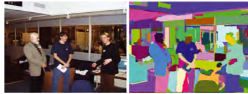
(d) Graph-Based Segmentation: color segmentation by graph-partitioning (taken from [Felzenszwalb and Huttenlocher, 2004])
