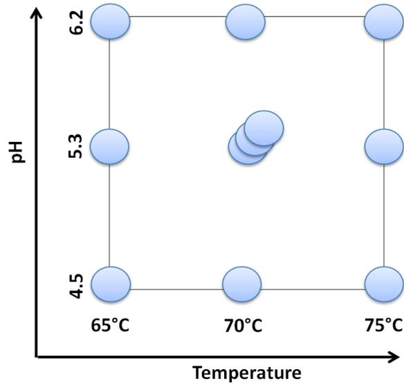
**Figure 9:** Illustration of experimental design space revealing the variation of temperature and pH, at which the x-axis indicates the different applied temperatures, whereas y-axis describes the used pH-values. Each circle represents an individual enzyme reaction, which was run at specific time points. In the middle of the design, the triplicate center points are positioned (70°C and pH 5.3).
