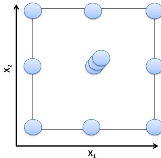
**Figure 8:** Illustration of a CCF design, which shows the to investigate experimental space in regard of two factors  $X_1$ ,  $X_2$ . Each of the represented circle stands for an individual experimental run at specific conditions. In the middle of the design, the triplicate center points are positioned, which are carried out to estimate experimental error.
