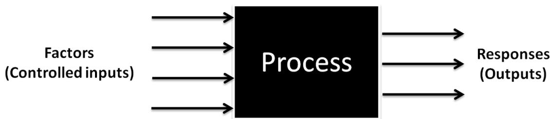
**Figure 7:** Schematically showing the black box process model characteristics of DoE. The applied factors and obtained responses of the specific process are mathematically related to each other. Adapted and modified from Mandenius et al. [69].
