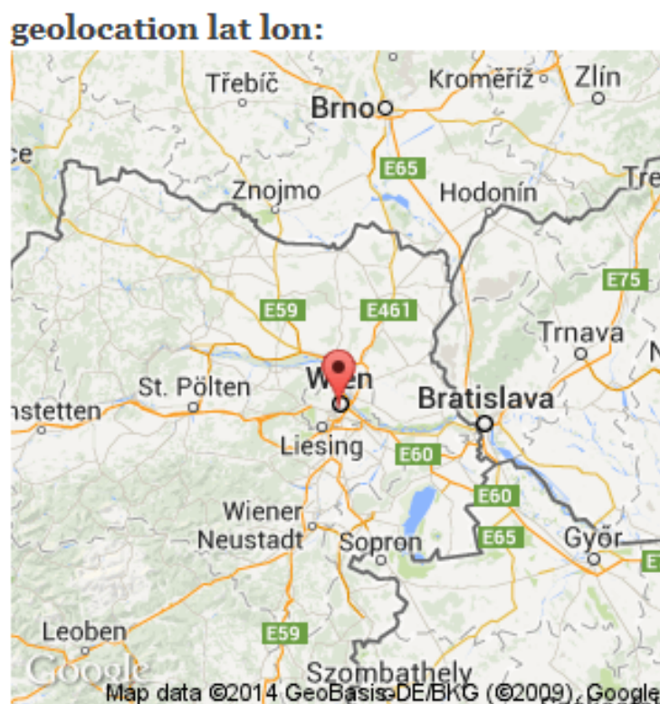
Figure 3.3: A generated static map jpeg file using the Google Static Maps API and the default settings in Drupal's Geolocation module.
