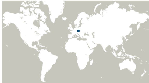
Figure 3.4: The default behavior in Chrome using the HTML5 Geolocation specification. A map is generated of the world and a blue dot signifies the position returned from the navigator object.
