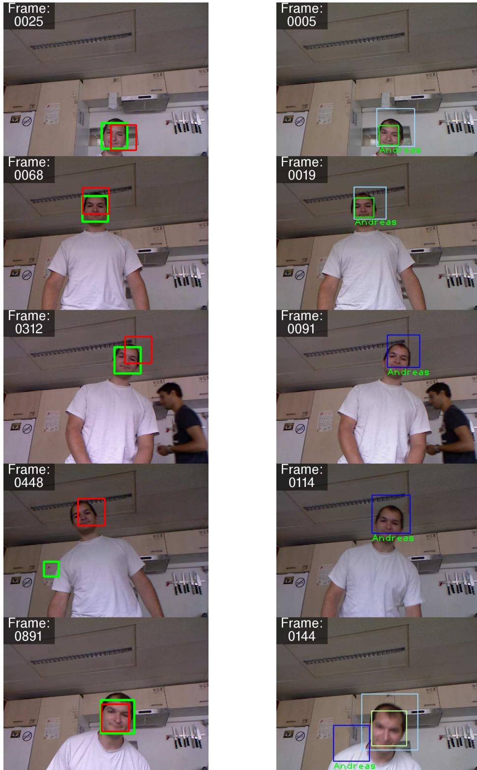
(a) 2D detection and Kalman filtered tracking
