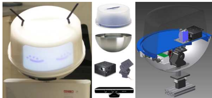
Figure 1.2: Eva - components and design. Source 1
