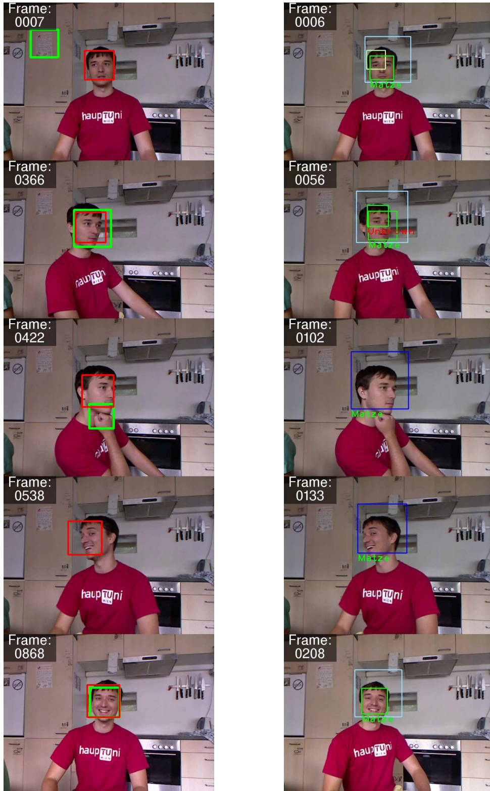
(a) 2D detection and Kalman filtered tracking
