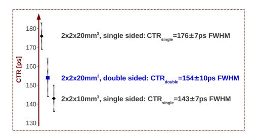
**Figure 9.8.:** Comparing single sided readout with double sided readout. The standard single sided readout measurements give 176ps FWHM CTR for 20mm long crystals. Whereas the time resolution improves to 154ps by using double sided readout of the same 20mm long crystal. In comparison 10mm long crystals readout single sided give a CTR of 143ps FWHM.
