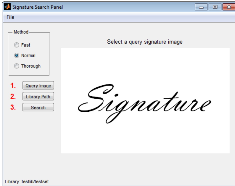
Figure 4.12: The main window of the prototype which allows to search signature image libraries with a query signature. The numbers on the left indicate the steps necessary in order to search a signature library.
