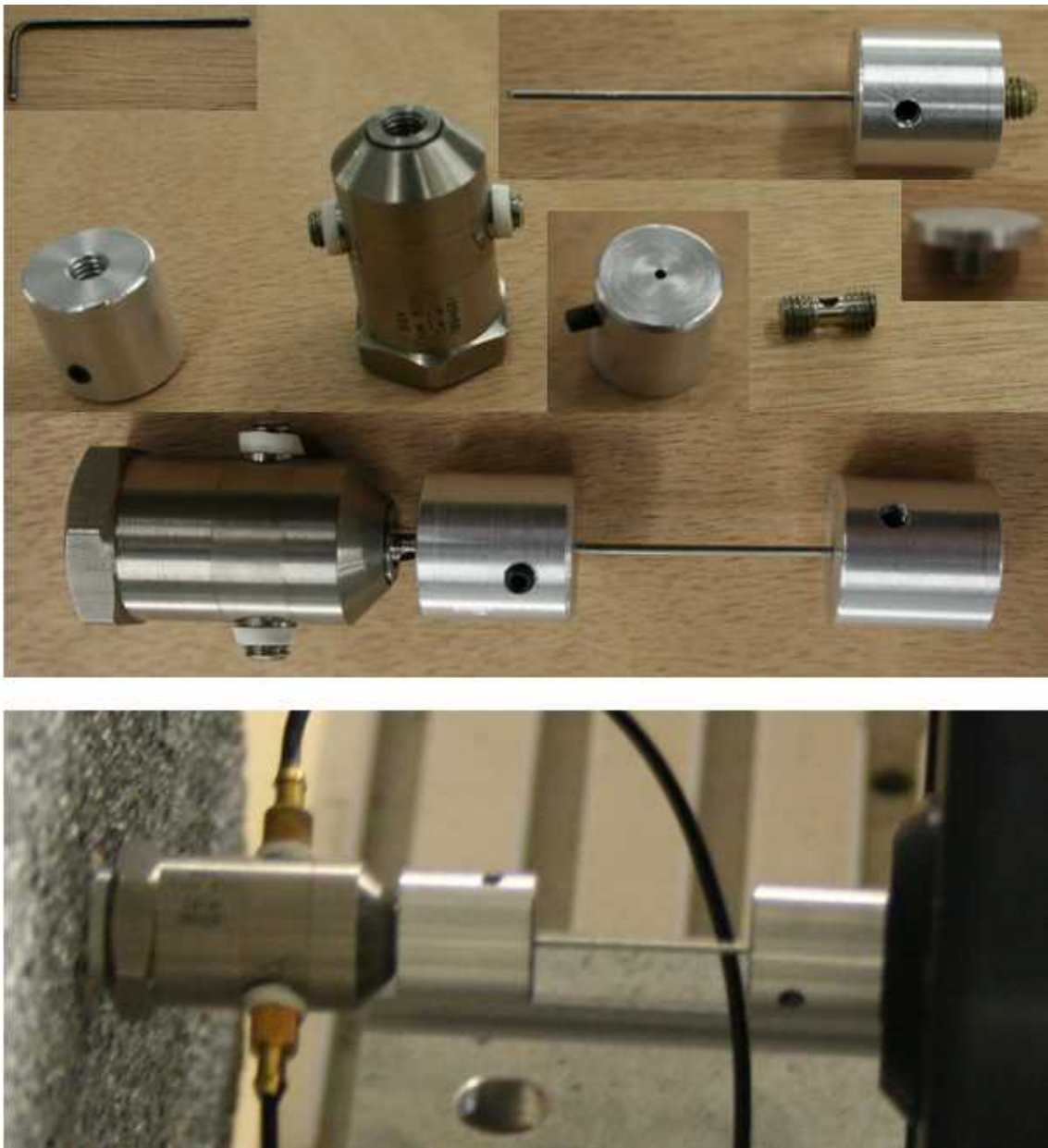
Figure 2.12 Shaker and structure attachment (Stinger assembly)
