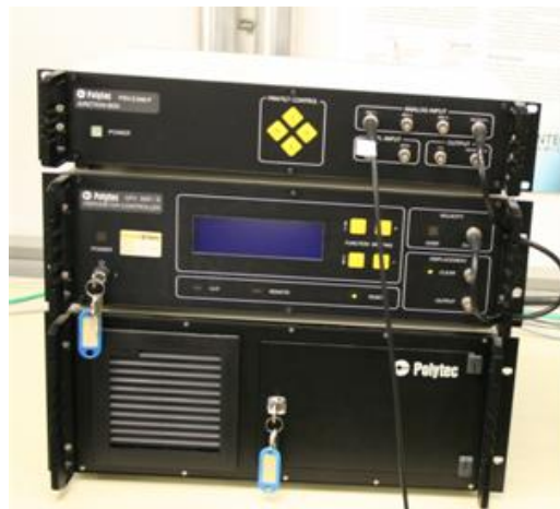
Figure 2.8 Polytec system components, work station, controller OFV-3001-S, junction box PSV-Z-040
