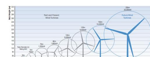
Figure 4: Growth in size of typical commercial wind turbines
