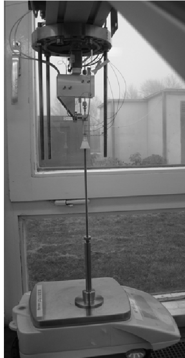
Figure 164 Calibration setup of the DM thrust stand
