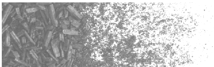
Figure 111 Close capture of pellets (left) and debris (right) of configuration #30 after accumulated hydrogen peroxide load of 360 g
