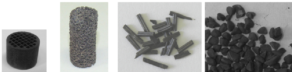
Figure 100 Catalyst of test campaign 2: from left to right: 304 cpsi monoliths of 10mm length (#23), foam of 20mm length (#28) and detail of pellets #30 and of milled pellets of conf. #38
