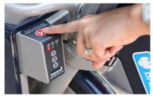
Figure 139: Device in the docking point used by customers to report damaged bicycles in the Barclays Cycle Hire of London (Georgiou 2010).
