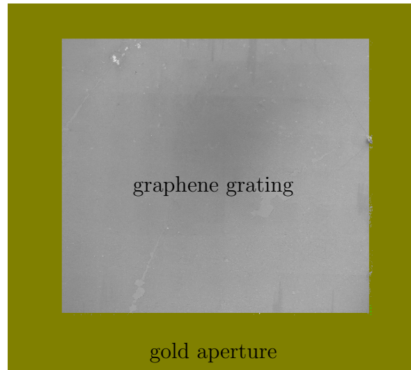
Figure 3.7: Scanning electron microscope picture of the fabricated grating with a gold aperture. The opening is 1.9 \times 1.9\text{ mm}^2 large.
