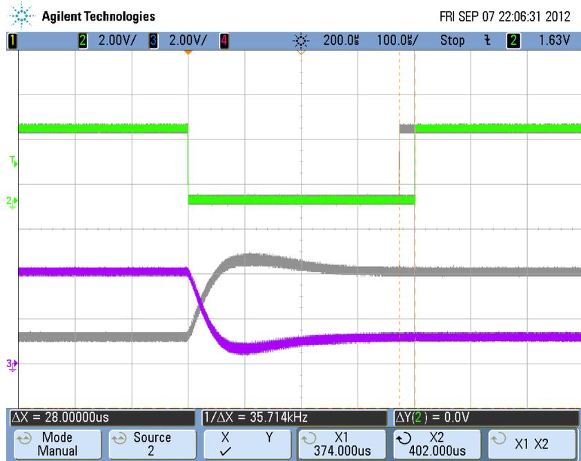
Figure 7.16: VCO1 switching between 1030 MHz and 1090 MHz (upper curves: lock detect, lower curves: tuning voltage)
