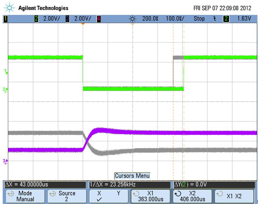
Figure 7.17: VCO2 switching between 1090.5 MHz and 1145 MHz (upper curves: lock detect, lower curves: tuning voltage)
