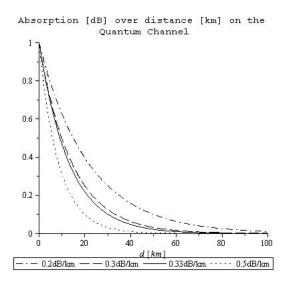
Figure 5.3: Maple Simulation of the Absorption on the Quantum Channel - d variable
