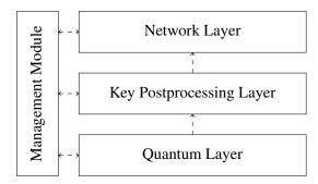
Figure 5.12: Layer Structure of Q3P
