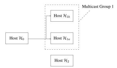
Figure 3.13: Multicast Addressing of IPv6
