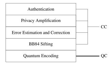
Figure 4.12: Protocol Flow of the Quantum Key Exchange
