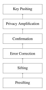
Figure 5.14: Protocol Stack of Quantum Key Distribution
