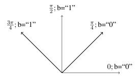
Figure 4.6: Bit Encoding of the Photon Polarizations Quantum Key Distribution
