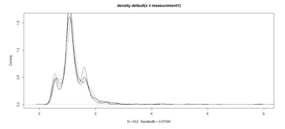
Figure 6.5: Latency Probability Density Function of IPv4
