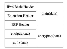
Figure 3.10: Structure of the Security Header of IPv6
