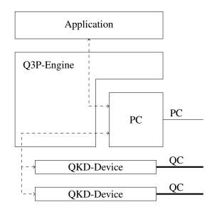
Figure 5.9: Network Node Structure of a QBNI in Q3P
