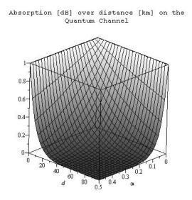
Figure 5.2: Maple Simulation of the Absorption on the Quantum Channel -  $\alpha$ , d variable
