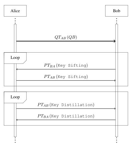
Figure 4.13: Sequence Diagram of the Primary Protocol Stages of BB84
