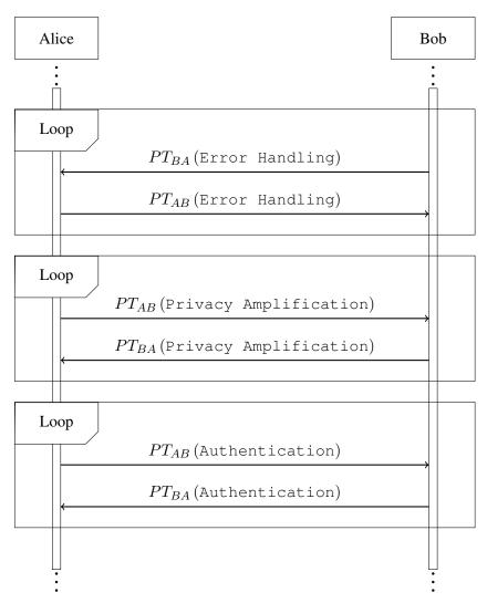
Figure 4.17: Sequence Diagram of the Key Distillation in BB84
