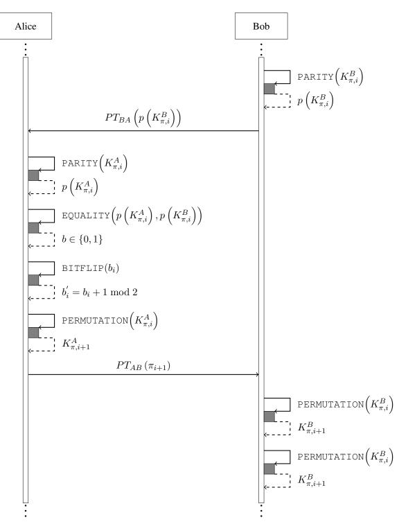
Figure 4.18: Sequence Diagram of the Transmission of parity bits over the Public Channel in the BB84 Error Handling
