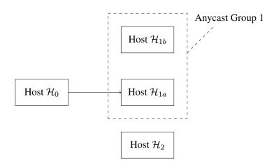
Figure 3.14: Anycast Addressing of IPv6
