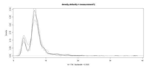
Figure 6.11: Latency Probability Density Function of Quantum Key Distribution (Q3P)
