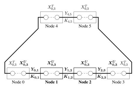
Figure 5.10: Transmission of a Quantum Key over a QBNI with k = 2 < n untrusted nodes -  $K_{final} = (X_{0,3}^U \oplus X_{0,3}^T)$
