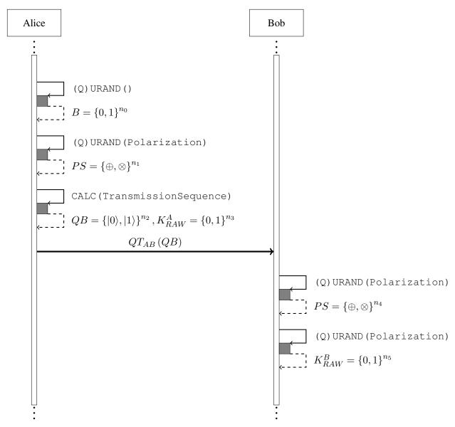
Figure 4.14: Sequence Diagram of the Quantum Transmission to obtain the Raw Keys  $(K_{RAW}^A, K_{RAW}^B)$  in BB84 -  $n_i \le n_{i+1}$
