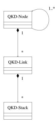
Figure 5.7: UML of the Node, Link and Stack associations in a QBNI
