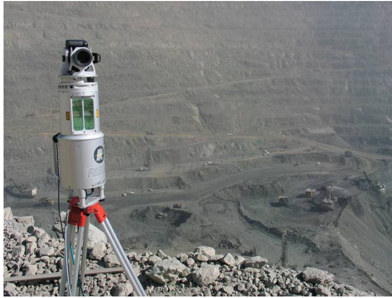
Figure 2.3: 3D range scanner with a mounted camera [20].
