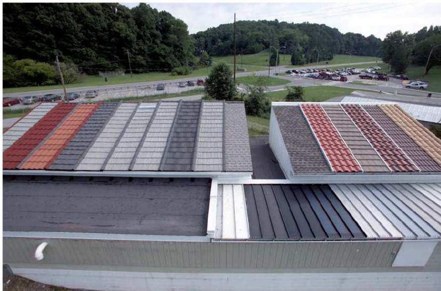
Figure 10 ORNL's roof study in Florida (Miller et al.)
