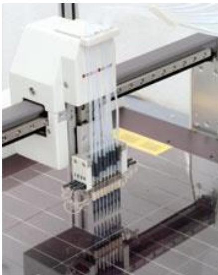
Figure 4: Print head for non-contact spotter. Small droplets of protein solution are fired onto the microarray slide surface. Image from Eisenstein [109].
