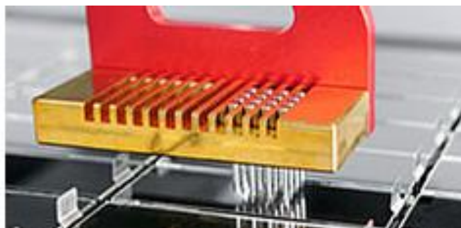
Figure 3: Print head of contact spotter. Capillary pins arranged in the allotted slots are used for the deposition of protein solution onto the microarrays. Image from Arrayit corporation.
