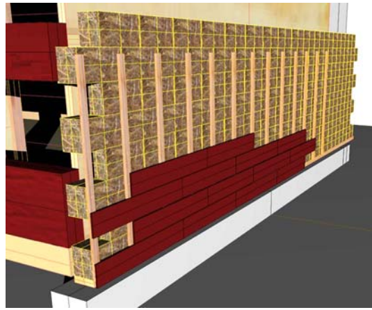
9.3.8 clt panel with straw bale + ventilation
