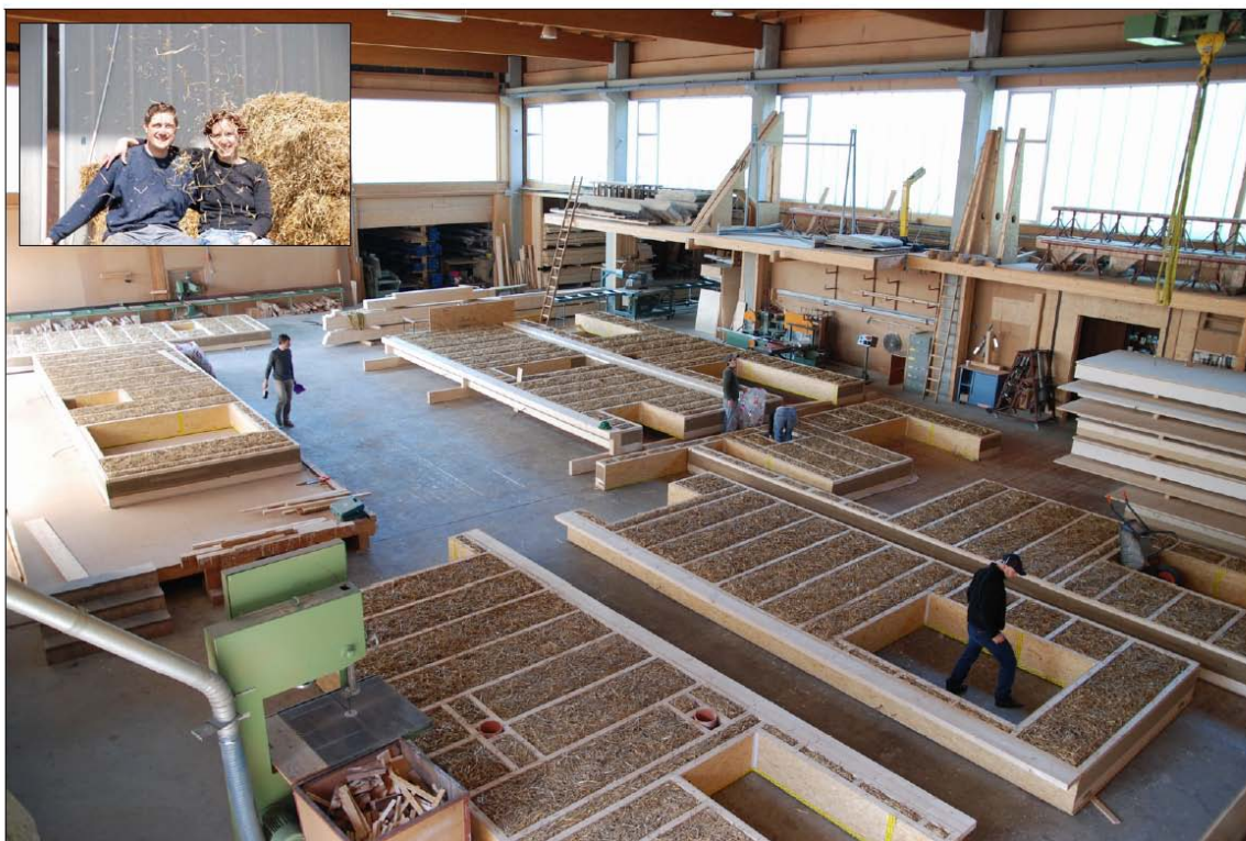
9.3.1 prefabrication of wooden framework with strawbale-infill; [23] www.fasba.de
