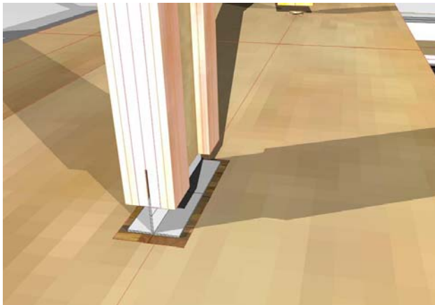
9.6.6 bearing plat and post connection
