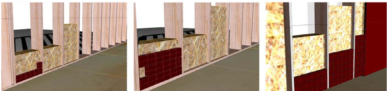
9.6.4 layers of the outer courtyard wall
