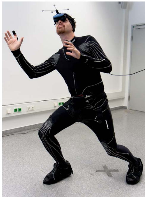
Figure 62: The developed active motion suit in combination with a passively tracked head mounted display.
