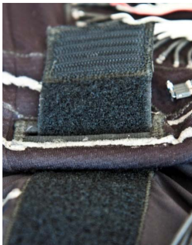
Figure 43: Four of these loops are mounted on the trousers and can be pulled through slots in the shirt.
