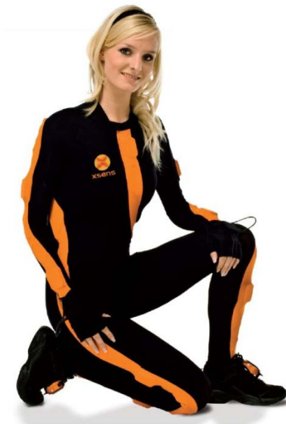
Figure 5: Xsens “MVN” is an inertial motion capture solution (courtesy of Xsens).
