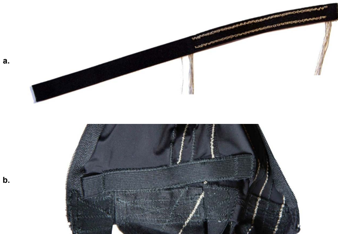
Figure 48: Bridgeover for Joint LEDs a. Before and b. After Mounting
