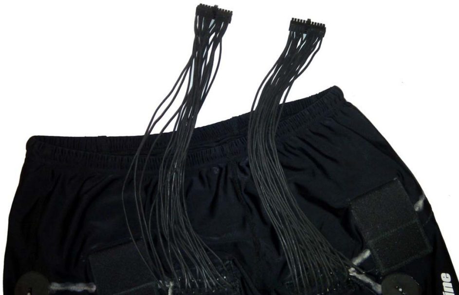
Figure 49: Cables of Conductive Thread with Heat Shrinkable Tubing as Insulation
