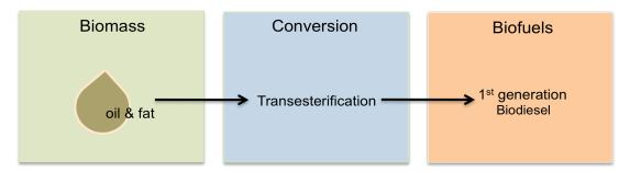
Figure 6: Schematic conversion process for 1<sup>st</sup> generation biodiesel
