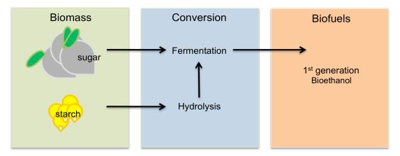
Figure 4: Schematic conversion process for 1<sup>st</sup> generation Bioethanol
