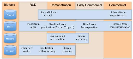
Figure 11: Development status of the main technologies to produce biofuels for transport from biomass
