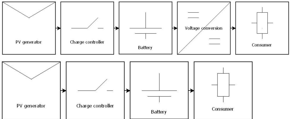
**Figure 1: Schema of an off-grid PV system without and with voltage conversion**
