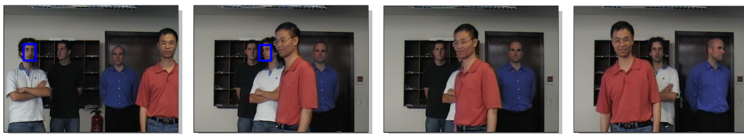
Figure 2.3: Recursive tracking is possible as long as the selected object is visible in the image. In the third frame an occlusion occurs. Images are from the SPEVI 1 dataset.
