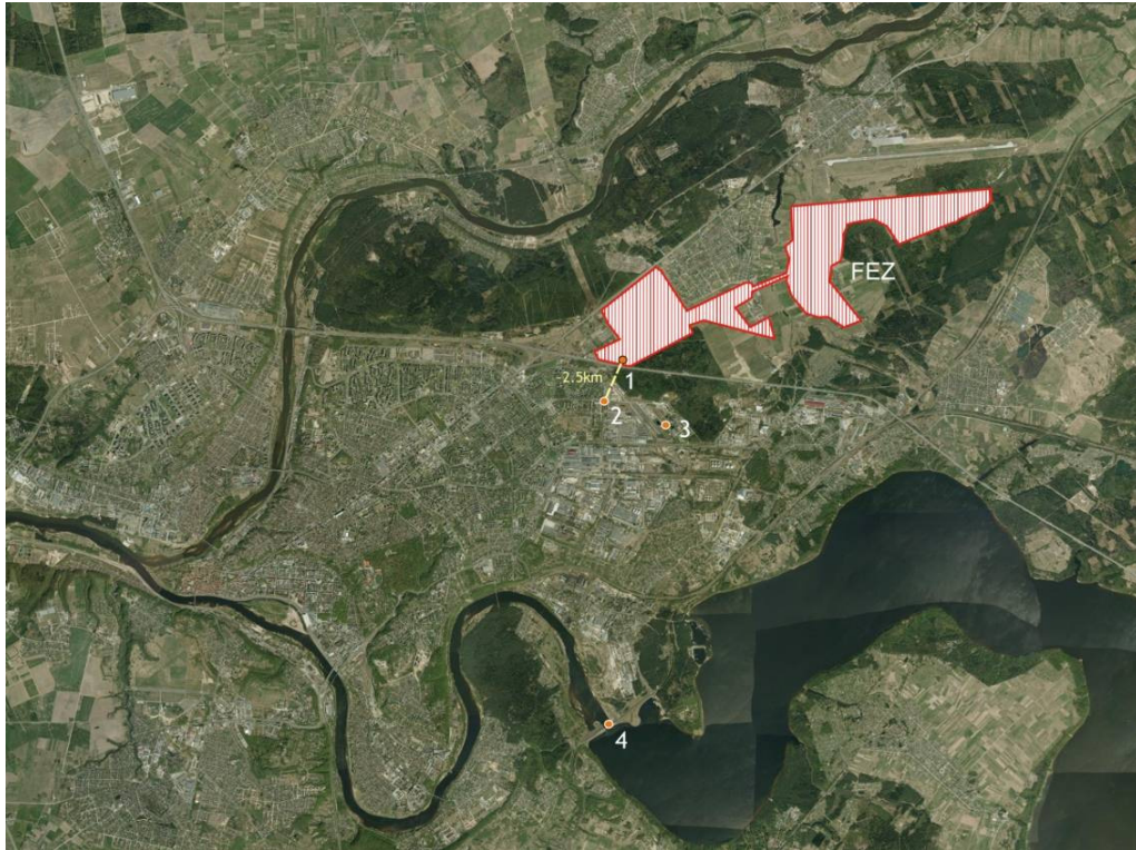
Figure 5-1 Implantation of biomass CHP plant and connection possibility to Kaunas district heating network
