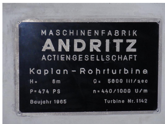
Figure 7: Nameplate of turbine
