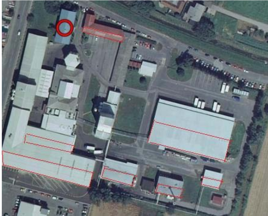
Figure 67: Red lines on the satellite image mark surfaces for solar energy use (Engis.si)
