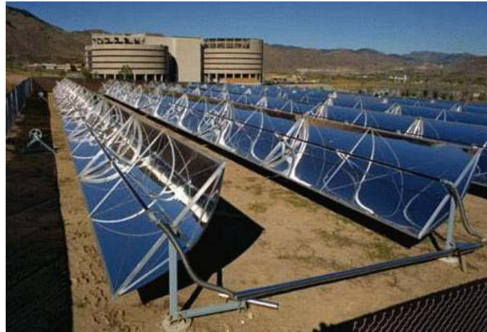
Figure 21: Parabolic trough concentrators (NREL)
