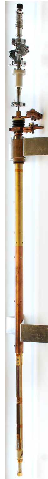
Figure 3.16.: 1000 A sample rod used for transport measurements. (a) Design drawing (broken at three points to keep the aspect ratio reasonable). (b) Photograph.
