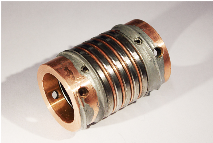
Figure 2.3.: Wire sample for transport measurements mounted on a Ti-6Al-4V barrel equipped with copper rings for electric connection.
