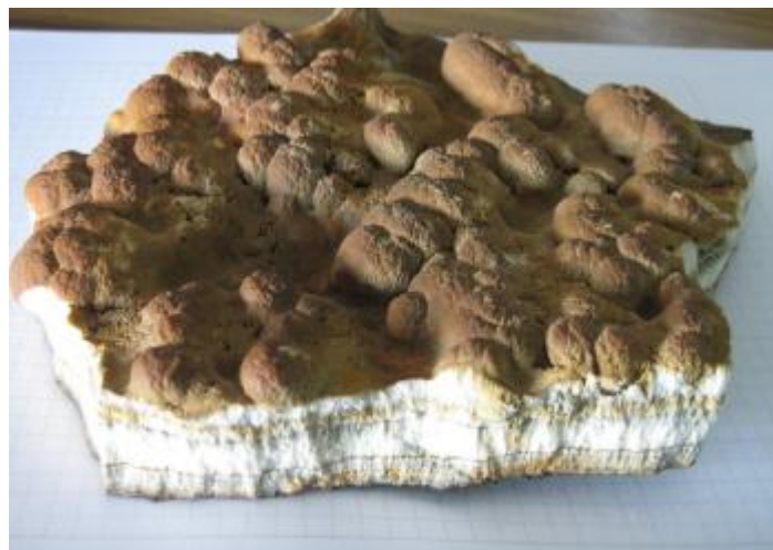
Figure 13: Scale formed in the Surface Plant at Soultz
