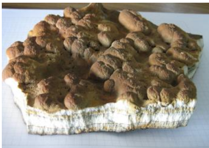
Figure 5: Sample of scale that forms in the Soultz installation
