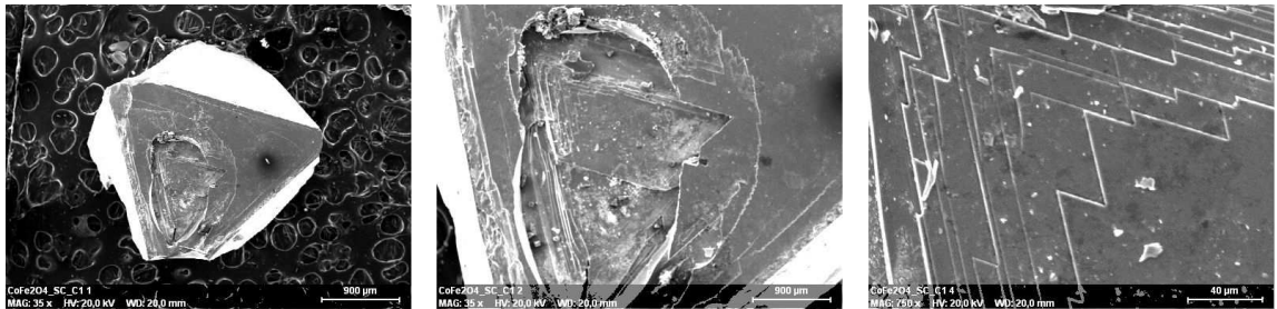
Figure 5.1: Triangular (111) plain of the as grown, octahedron shaped Cobalt Ferrite single crystal
