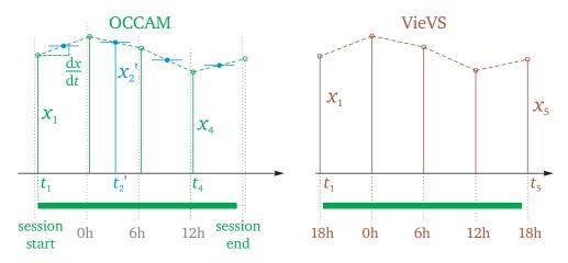
Figure 4.2: Setup of time dependent parameters in OCCAM and VieVS.
