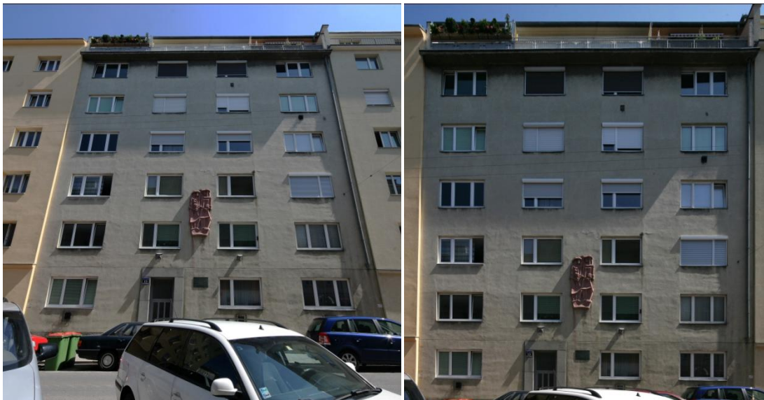
Fig. 4.9 Facade image from 1,5m height shot with Canon TS-E 17mm (left); facade image from same position shot with Canon TS-E 17mm using the shift functionality (right)
