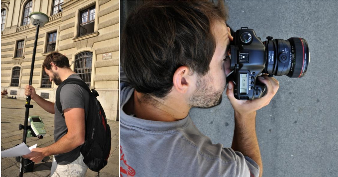
Fig. 4.5 Measurement of GPS reference points (left) and photography with Tilt-Shift lens (right)
