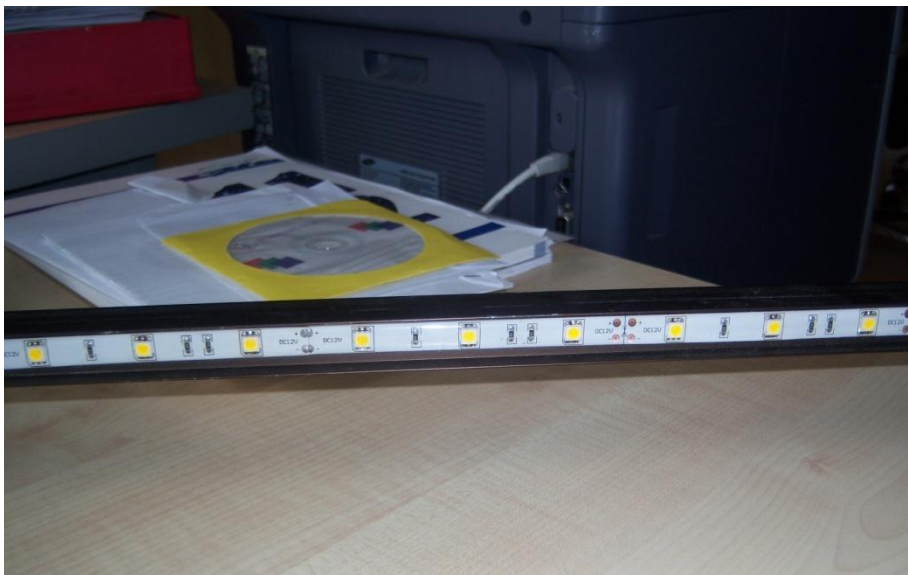
Photo 6. LED strip in the lamp with SMD LED 5050
