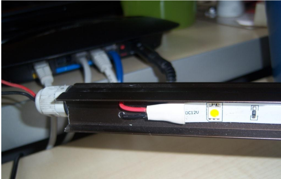
Photo 5. Detail showing ending with heat shrinkable tubing and cable entry
