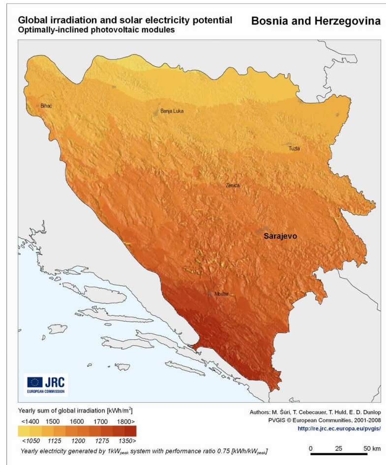
Figure 7. Yearly sum of global irradiation and yearly electricity production potential for optimally inclined, south facing, PV modules in Bosnia and Herzegovina (PVGIS, 2012).
