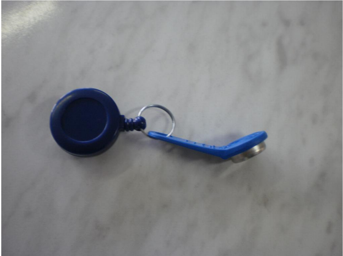
Fig.16. iButton device used for driver login function.
