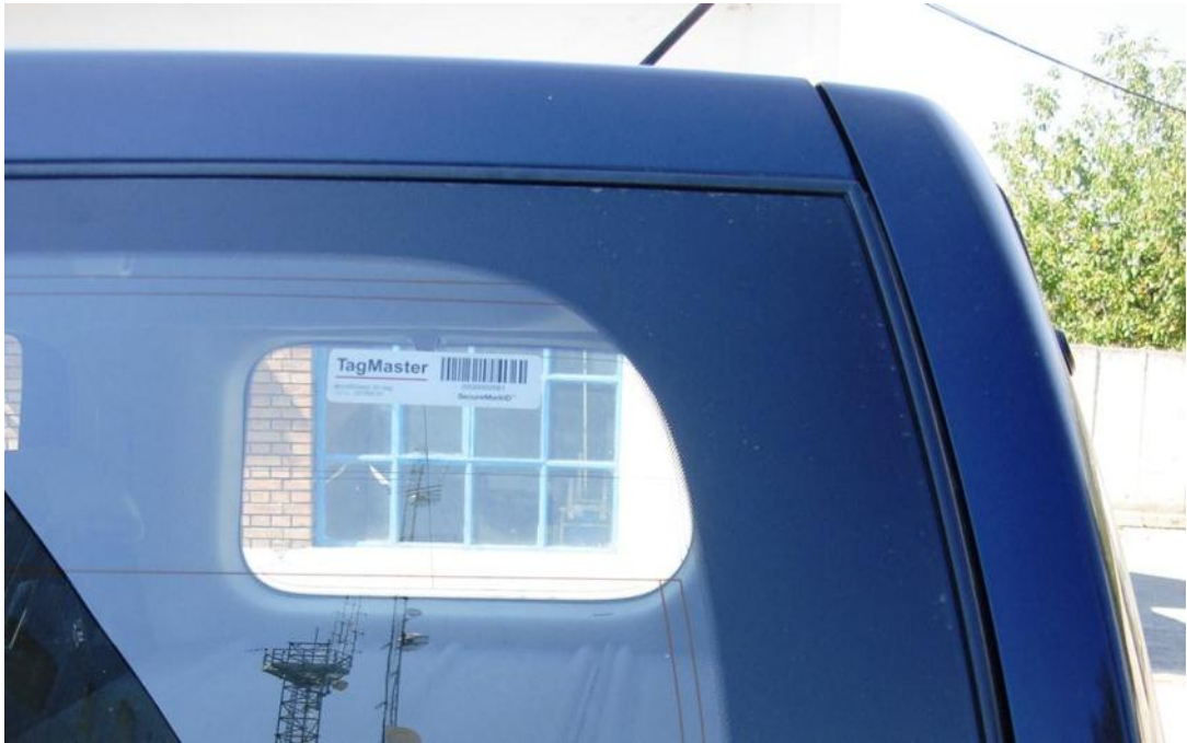
Fig.17. RFID tag installed to the vehicle
