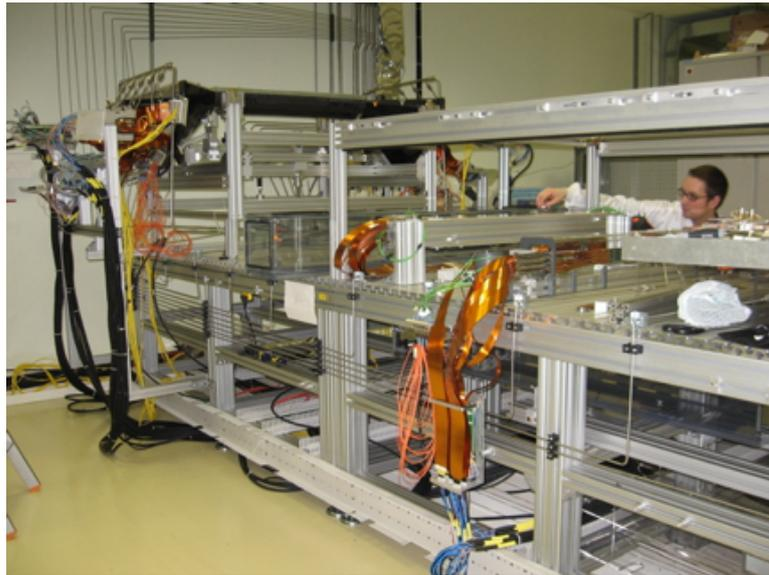
Figure 4.3: Test bench in the clean-room at CERN. In foreground 2 sectors are mounted, in the background the first half-barrel is mounted.
