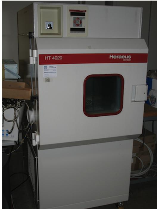
Figure 3.24: Heating chamber used for the cycling tests.
