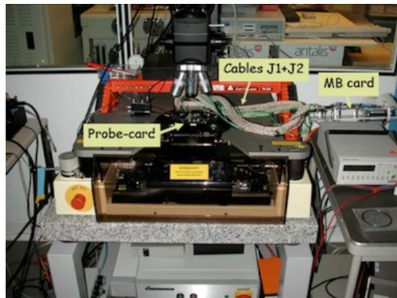
Figure 3.11: The SÜSS probe station at CERN. The probe card is connected via cables J1 + J2 to the DAQ adapter board. The voltage supply to the chip is provided via the DAQ adapter board. The bias voltage is supplied via a needle which is connected to the back-side of the sensor [36].
