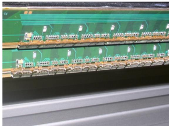
Figure 4.6: Picture taken during a visual inspection. It is important to find any damage on the sector before switching on. For instance bended wire bonds would cause short circuits.
