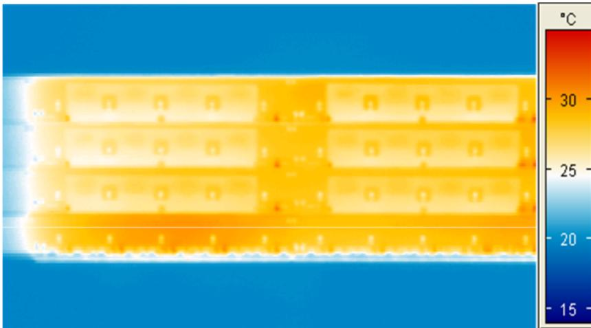
Figure 4.2: Infrared picture of the outer layer of an half sector during operation.
