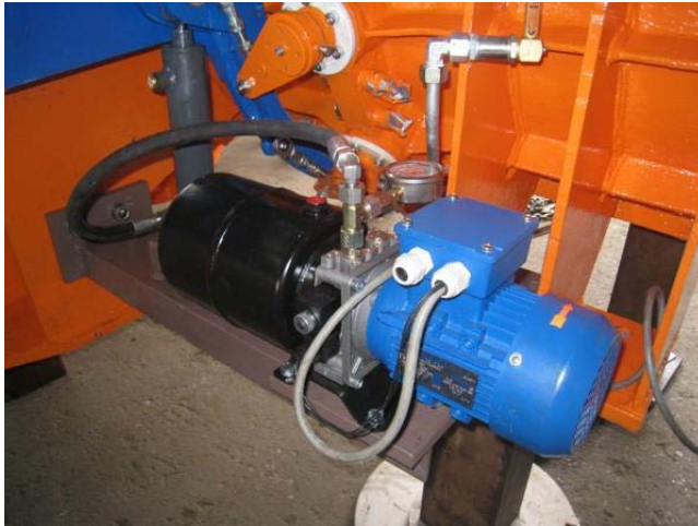
Graph 24: Hydraulic Aggregate with Cylinder for the Wicket Gates
