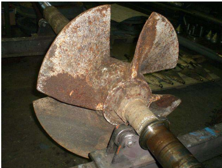
Graph 19: Runner in old Status, with welded Runner Blades, strong Corrosion
