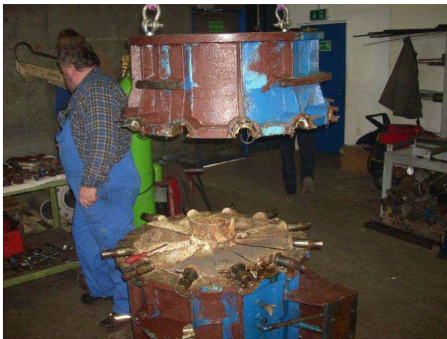
Graph 23: Disassembly of the Casing
