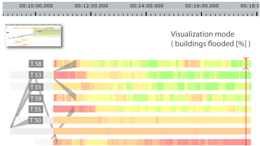
Figure 2.24 – Visualization mode that analyzes the percentage of flooded buildings using a combined current time-step and frame-wise visualization of all tracks that were investigated during the refinement and stability-test stages.
